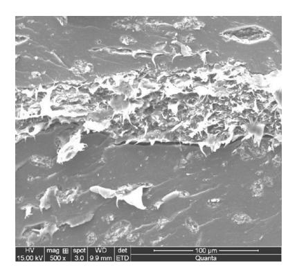
SEM micrograph of fractured surface with 5% NC
