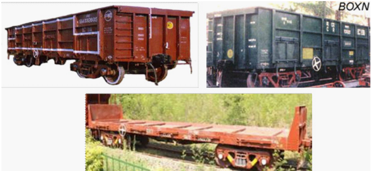
Figure 20: Key wagons used to move steel by Indian Railways (Clockwise from top left: BOST, BOXN, and BRN) Source: IRFCA
