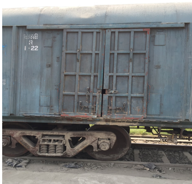
Figure 23: Ill-fitting wagon doors lead to product damage during transit
