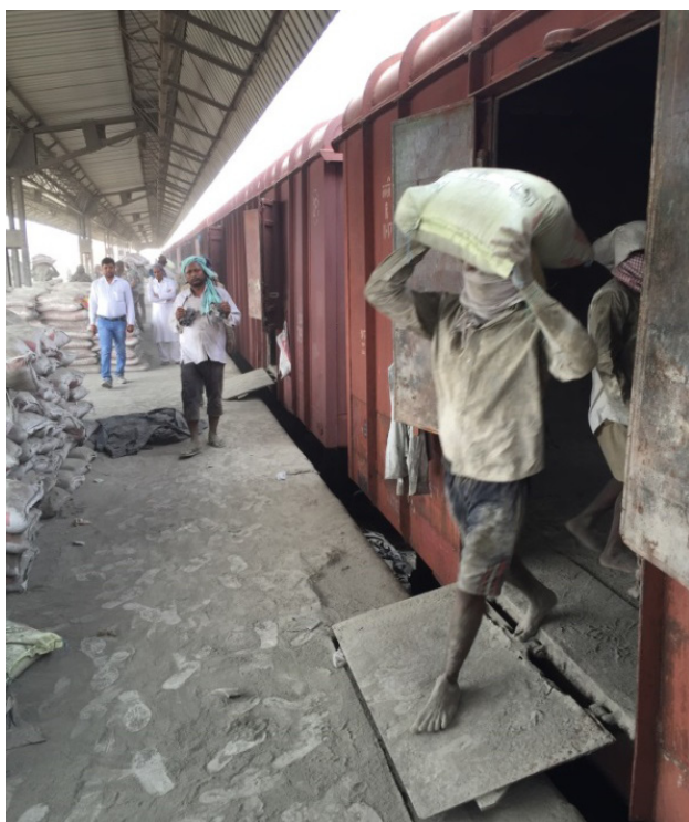
Figure 21: Lack of suitable footwear, protective masks and accumulation of cement dust in the air and on the platform have major side effects for the workers Source: Site visit, TERI
