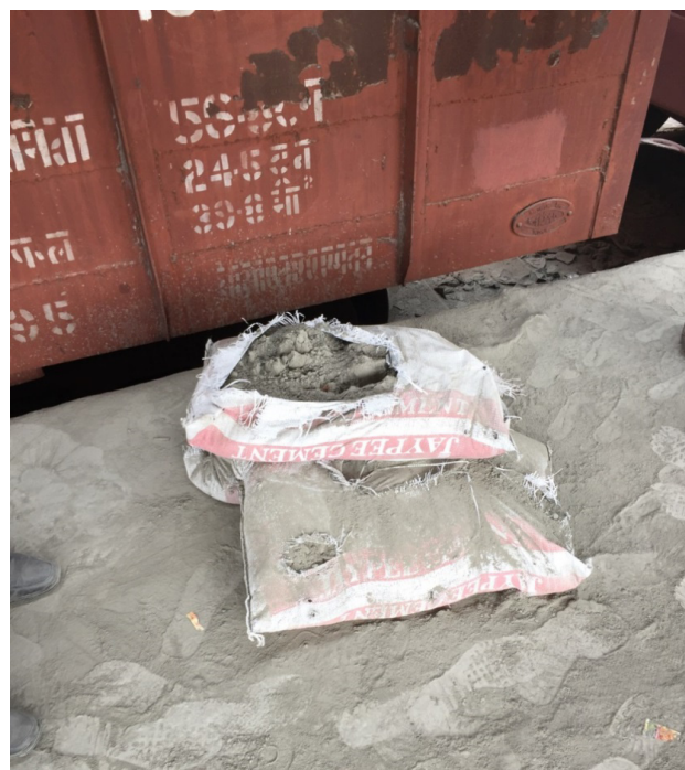
Figure 22: Split cement bags lead to a significant loss of the product Source: Site visit, TERI
