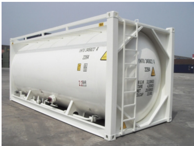
Figure 26: Cement tank for bulk movement of cement by either road or rail
