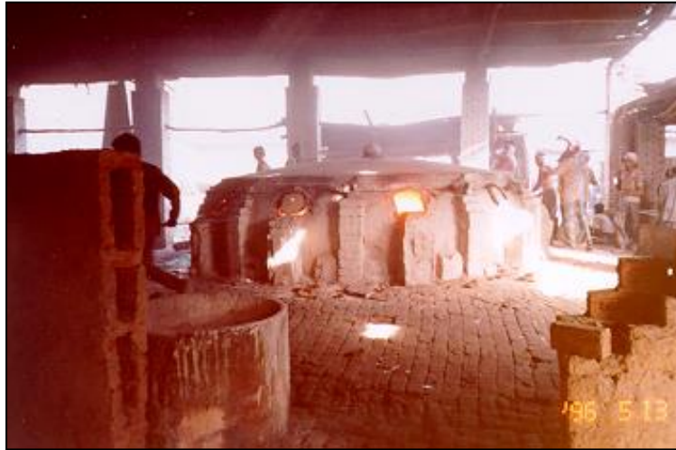
Conventional coal/NG fired Pot Furnace
