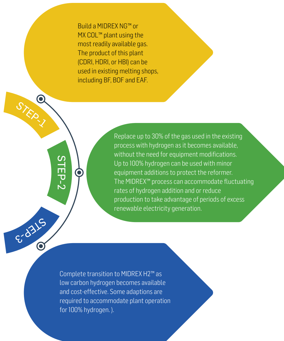
Figure 4: A stepwise approach to reducing CO 2 emissions via the direct reduction route
