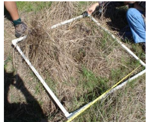
Wooden sampling frame for measurement of above ground biomass assessment (UNDP 2014)
