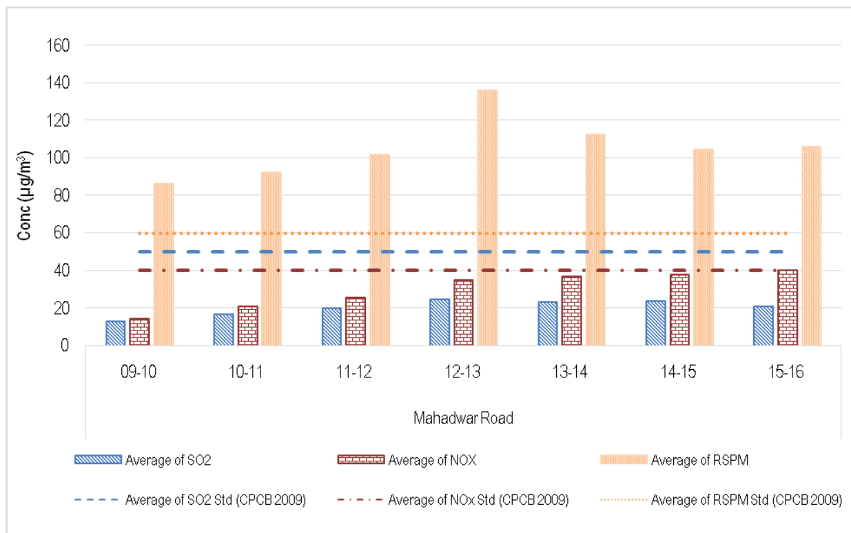
Figure No. 101: Annual average trend of SO 2 , NO x , and RSPM at Mahadwar Road
