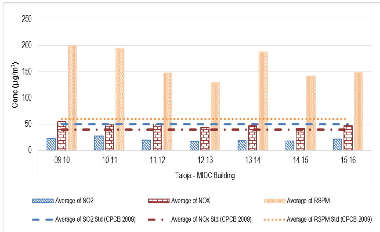
Figure No. 147: Annual average trend of SO 2 , NO x , and RSPM at Taloja - MIDC Building
