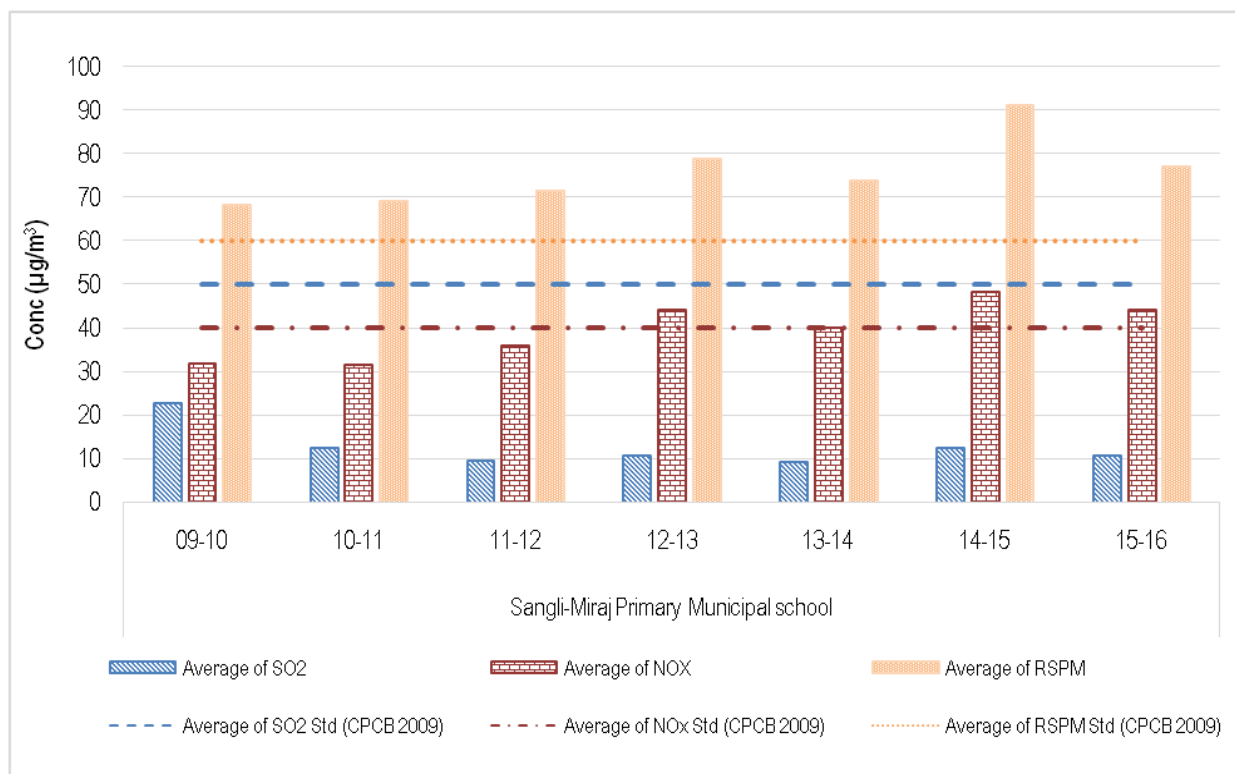
Figure No. 105: Annual average trend of SO 2 , NO x , and RSPM at Sangli – Miraj Primary Municipal School
