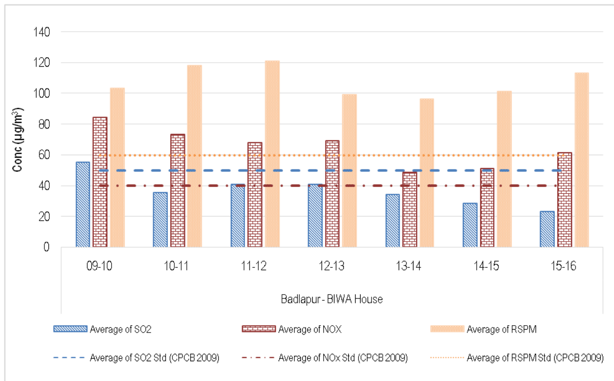
Figure No. 76: Annual average trend of SO 2 , NO x , and RSPM at Badlapur – BIWA House
