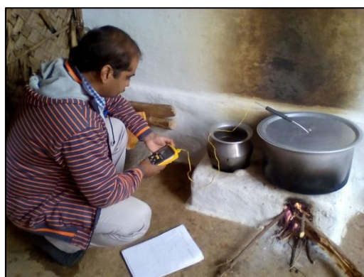
Picture 9: Thermal efficiency test conducted by TERI staff
