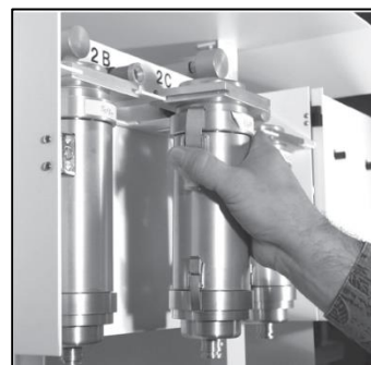
Fig. 2D: Chemcomb cartridge mounting in sampler
