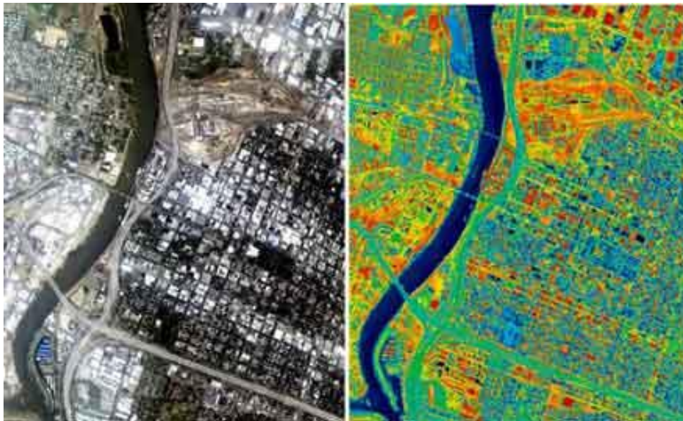
Figure 3-10 Thermal Image of a city showing temperature of different surfaces. (6)
