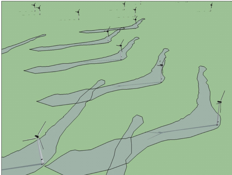
Figure A-VII.2 Shading of WEG-S82 at 10:00 am (21 st December) at Jakhau
