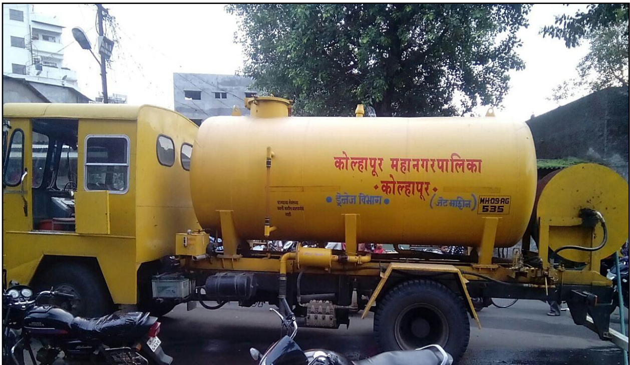
Picture No. 12: Truck mounted Jet Machine used by KMC Photo credits: Kolhapur Municipal Corporation
